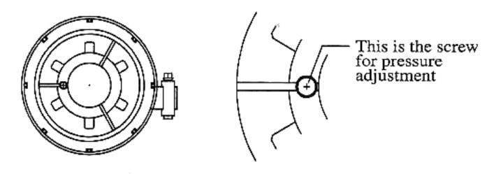
ATTN:To have proper adjustment, and be ware of the direction when install.
